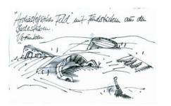
The courtyard of the BADER is build on the roof of a newly created underground car park. The carrying capacity of the ceiling did not allow sufficient soil replenishment for an extensive greening with bigger plants and so the task was to design an ,artificial landscape' as recreation area and play facilities for the residents and their children.
